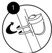
The transmitter unit should be mounted on the front side of the right fork blade, with the battery cover pointed upwards.
