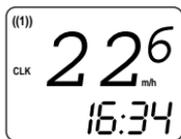
**CLK:** Clock with 12 or 24-hour display. Press the MODE button for two seconds in any mode to display clock. See - *To set the clock* (two paragraphs above) to program the clock.
