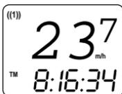
**TM:** Stopwatch. This function allows you to use the computer as a stopwatch. The stopwatch must be manually activated and stopped. The stopwatch records time regardless of whether or not the wheel is moving. Press the RED button to turn the stopwatch on and off.
