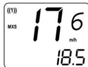
**MXS:** Maximum speed. This function displays maximum speed. Maximum speed is automatically reset when you reset the trip distance.
